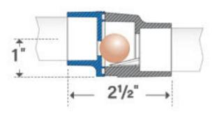
When condensate IS NOT present, the ball sets tightly against the seat.
