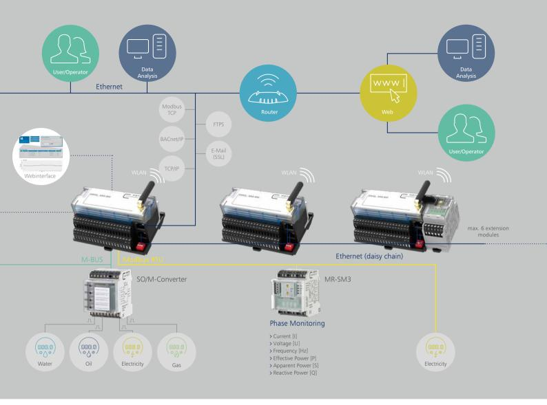
optional expansion modules for the conversion of physical properties such as temperature or S0 pulses into M-Bus telegrams, the collection of S0 double tariff meters, the expansion of I/O modules create countless expansion options for the system around the  $EWIO_2\text{-}M.$
