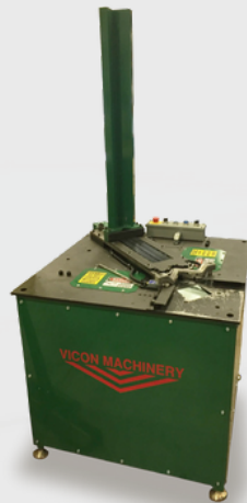
Single Head Corner Inserter Heavy duty frame structure designed for single corner insertion of flanged duct fittings. Machine utilizes various brands of TDX™, TDF™, TDC™ stackable corners. Standard tooling designed for 16-26 gauge duct.
